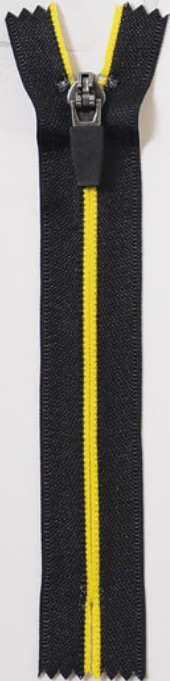
#3 Coil WR O/E zipper N39 semi-A/L slider U shape top stop Metal pin& box Puller: 90080 with reflective film Dull WR Tape Black
