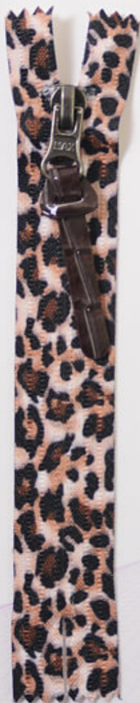
#5 Reverse Coil C/e zipper N51 MAX(T) A/L slider U shape top stop Welded bottom stop Puller: L0066 Heat Transfer Tape-HT-AZ
